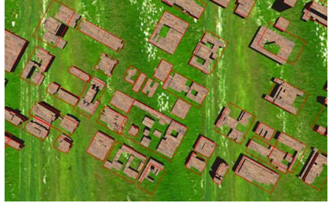
Figure 8. Base-buffer allocation. Each edge of the red rectangles denotes a base buffer.
