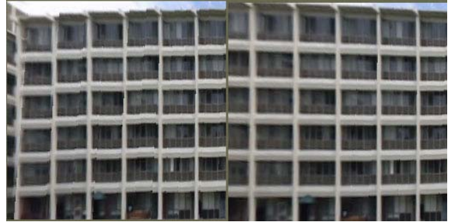
Figure 5. Refining texture alignment. Left: video painting using only 3D model-based warping, which results in significant misalignment due to an inaccurate camera pose. Right: video painting after refining the texture alignment.
