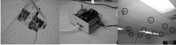
Figure 6: Bridged Hybrid Mica-Z on a Stargate (center) and Mica-Z on a PC (flanks) Test Bed
