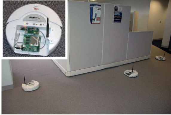
Figure 1: This photo shows a team of iRobot Creates, the platform used for physical tests of our algorithms. A more detailed view of the robot is shown in the inset.
